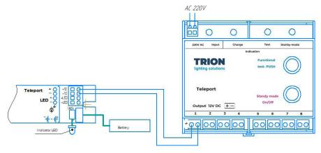
The length of the cable in the control circuit depends on the cross-section of the control cable and the number of connected lighting devices, data is shown in table 2.
